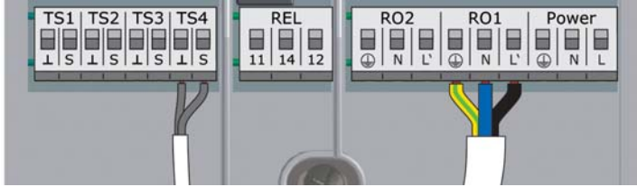
TS4: PWM-control signal for high-efficiency pump Left-hand terminal: GND Right-hand terminal: Signal
